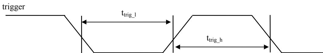
Figure 5-2 Hardware Trigger Timing
