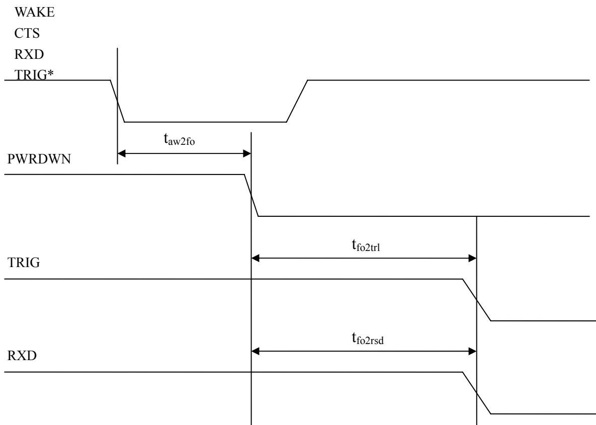
Figure 5-3 Wake up Timing
